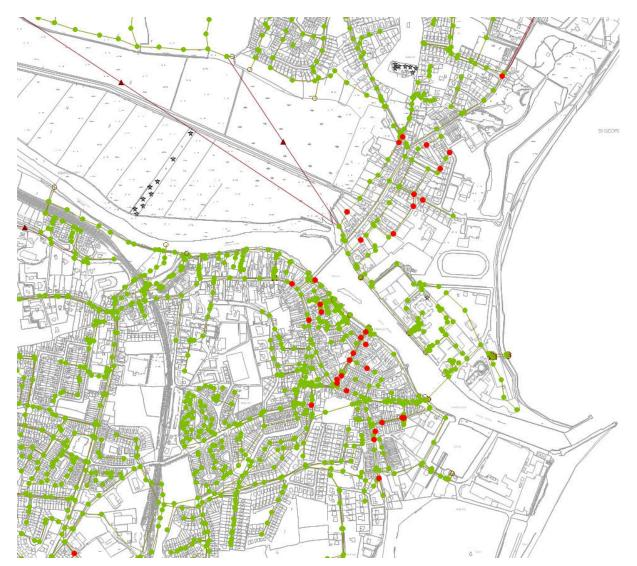
**Figure 6** Predicted flooding locations with flood volume >  $25 \text{ m}^3$  with all pumps down for M30\_60 & MHWS with CC
