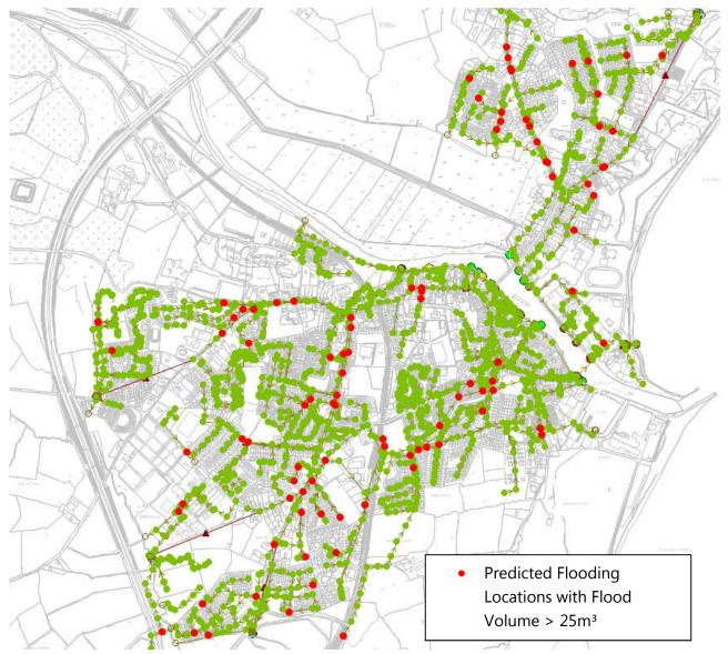
**Figure 2:** Existing System with Interceptor Sewer - Predicted flooding location > 25m3 for M30\_60 & MHWS with CC
